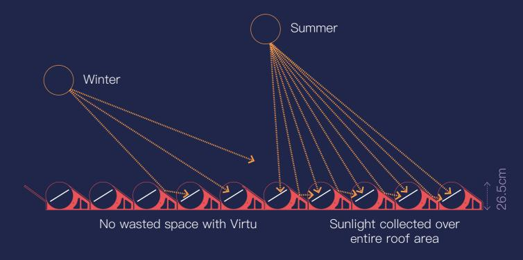
Not to scale. Virtu stands at 26.5cm high, compared to over 1m for tilted flat panel
