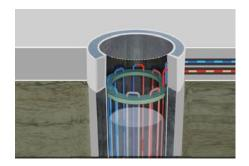
The patented Hiperpile utilises the high thermal capacity of the water-filled void to store thermal energy in the short term and exchange heat energy with the ground in the mid to long term.
