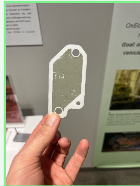
New Solid Oxide Fuel Cells tested on Mars to produce Oxygen from the Martian atmosphere.
