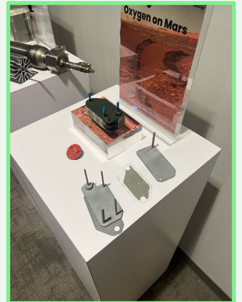
New Solid Oxide Fuel Cells tested on Mars to produce Oxygen from the Martian atmosphere.
