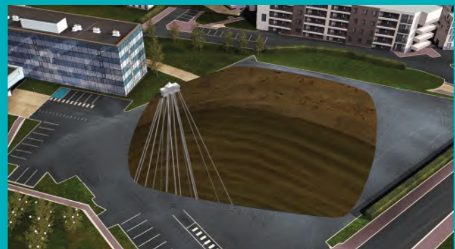
Illustration of the small footprint of the 10 geothermal wells in a star-shaped arrangement designed by Celsius Energy for this project.
