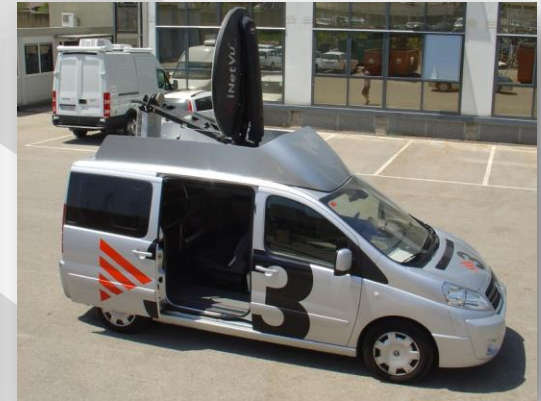
2010 – Driveway IP satellite connection
