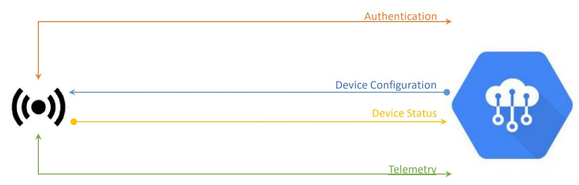
Periodically the gateway device on premises will collect the data for the pointset defined in the device configuration metadata and publish this to the MQTT topic '/devices/{device-id}/events/pointset'
