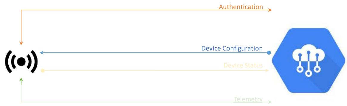
When a device attaches the Configuration previously provisioned on the cloud side is published to the 'config' topic
