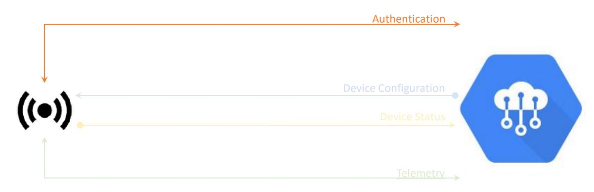
Connect to MQTT bridge/broker using TLS authentication and encryption using a JSON Web Token
