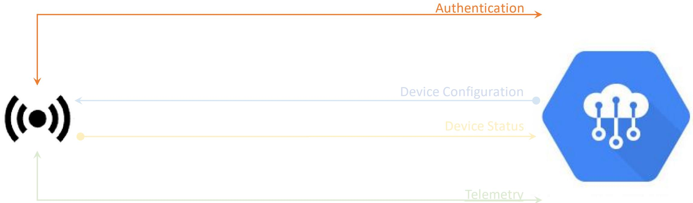
Connect to MQTT bridge/broker using TLS authentication and encryption using a JSON Web Token
