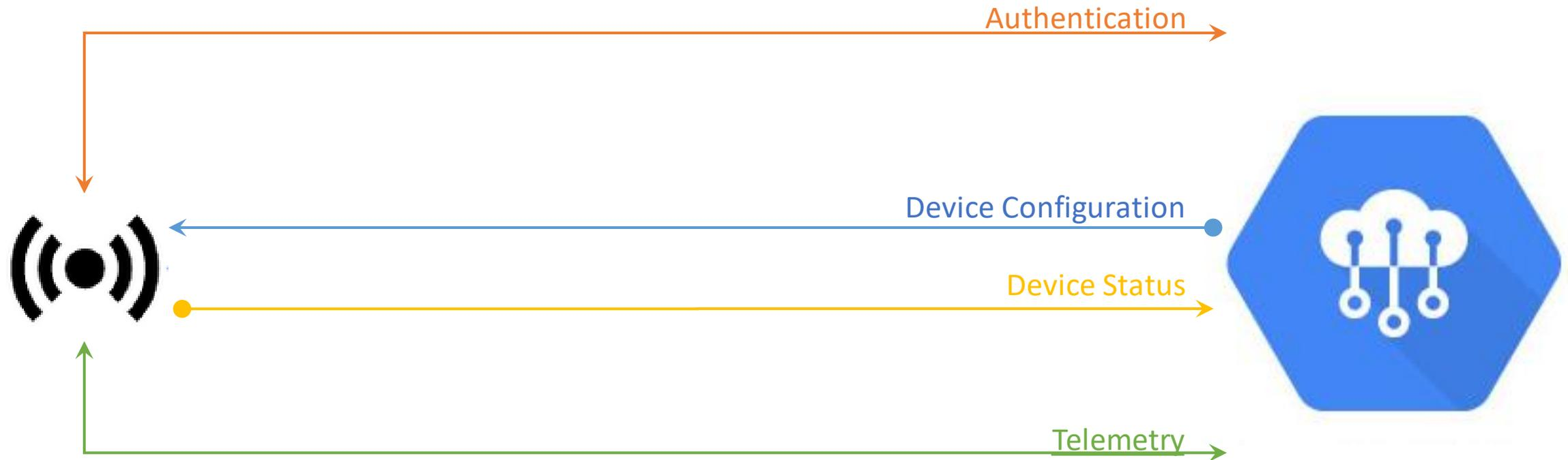
Periodically the gateway device on premises will collect the data for the pointset defined in the device configuration metadata and publish this to the MQTT topic `‘/devices/{device-id}/events/pointset’`
