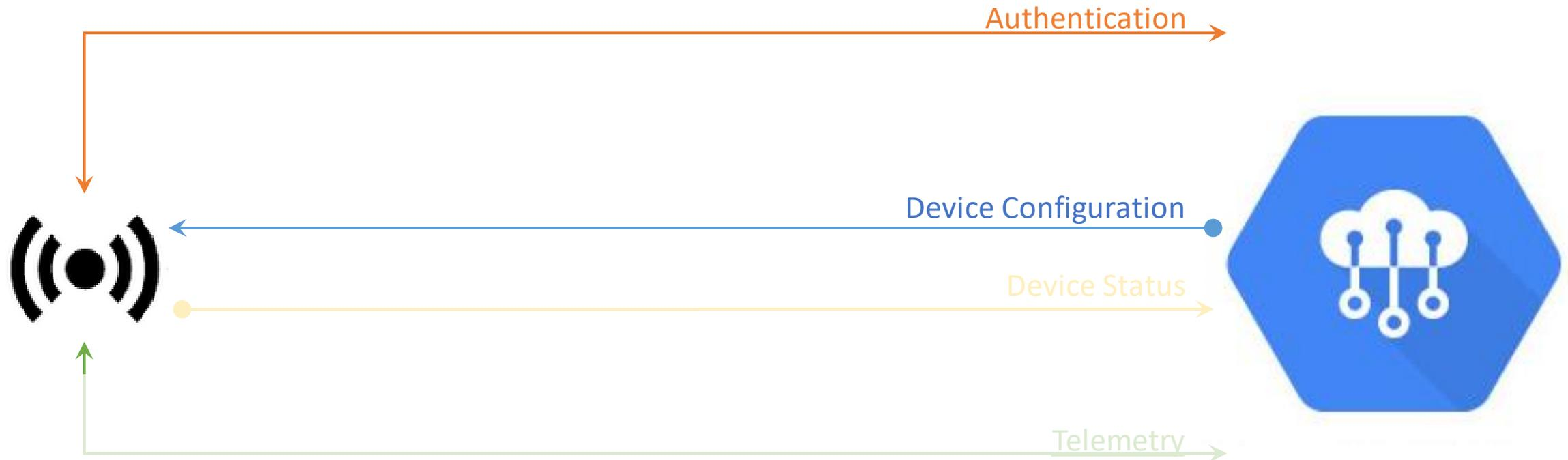
When a device attaches the Configuration previously provisioned on the cloud side is published to the 'config' topic
