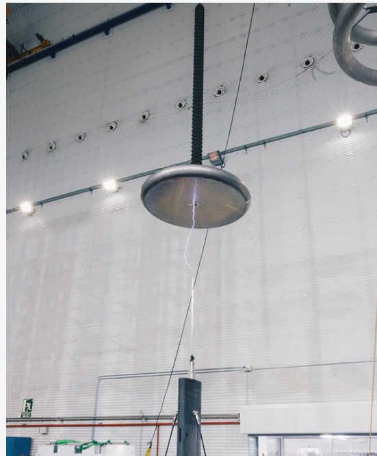
One of the high energy lightning strike tests that were carried out to evaluate a wide range of lightning protection systems.
