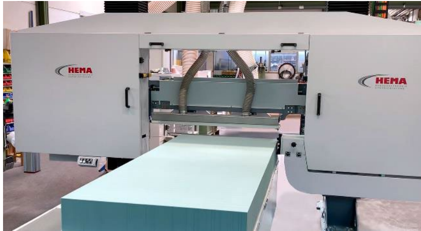
HEMA CoreCutter 900 for cutting PET rigid foam.
