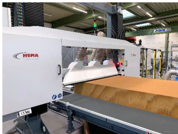
HEMA CoreCutter 900 for cutting aramid honeycomb blocks.
