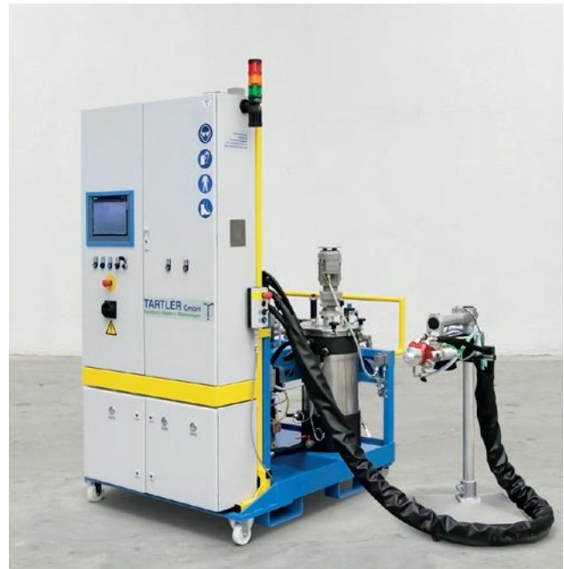
„Mixing is possible“: The new MDM plus from TARTLER bridges the gap between the company's portable small-volume systems and its large Nodopur systems (Fig.), which meter and mix up to 50 liters of resin per minute.
