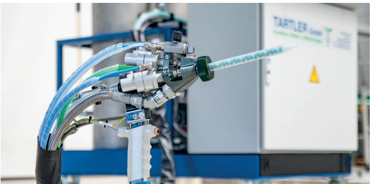
The new MDM plus from TARTLER is equipped with a LC5/3 mixing head. It can be fitted with disposable rotating plastic mixers – eliminating the need to use liquid rinsing agents.
