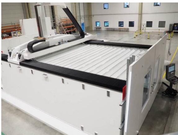
Fig. 3: The machine is still in Neuhausen. In Oberpfammern, Schröter will be able to machine complete vehicle models from five sides in a single setup.
