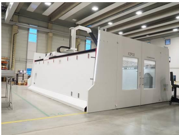
Fig. 2: The FZP32 5-axis portal milling machine is very accurate thanks to its thermosymmetrical design. It offers high productivity and availability.
