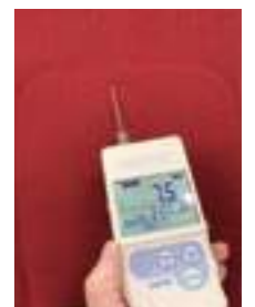
Measuring odor strength
