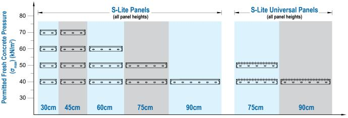
Panel Width of the S-Lite Formwork
