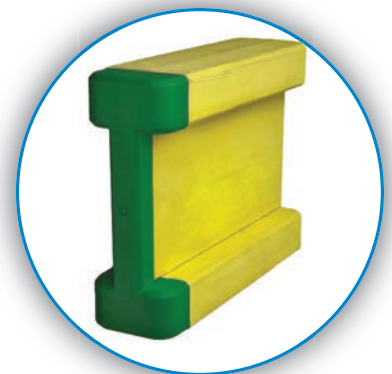
H20 Timber Beam Moment of resistance: 5.00 kN.m Shear resistance: 11 kN
