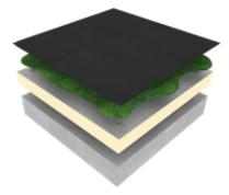
**FULLY ADHERED SYSTEM** The membrane is fully adhered directly to the substrate using Elevate bonding adhesive.
