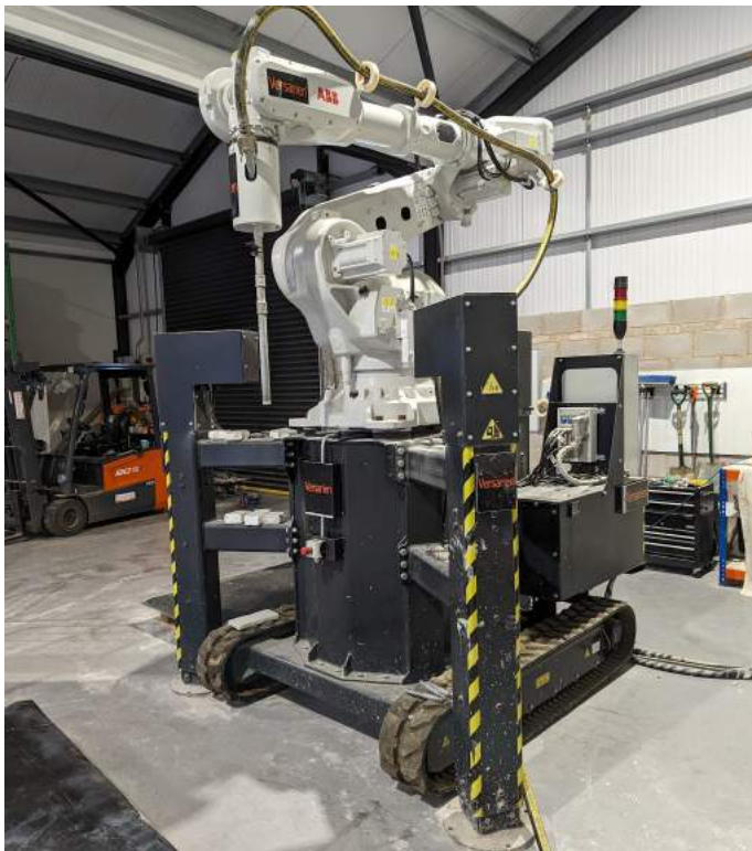
Versarien's robotic arm for 3D concrete printing.
