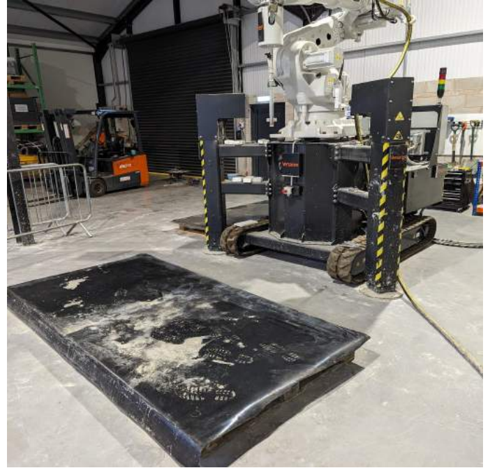
Print platform to ensure level and even print surface
