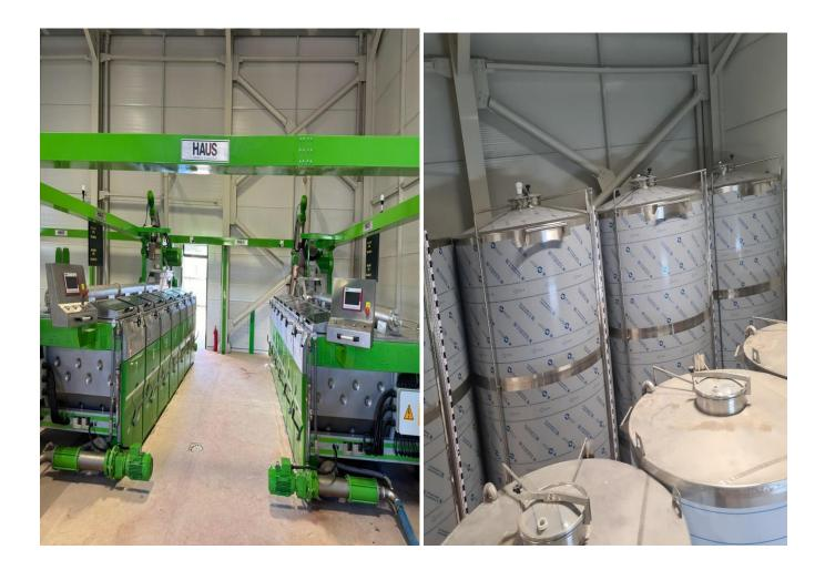
Once filtered by natural procedures, the new oil is transferred to our cellar where it will rest in small stainless steel tanks in an inert atmosphere thanks to the use of nitrogen and maintained at a constant temperature by means of an innovative air conditioning system.
