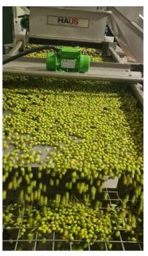
**Crushing:** The cleaned olives are transported to the crusher with an automatic conveyor. The crusher transforms the incoming olives into pulp.
