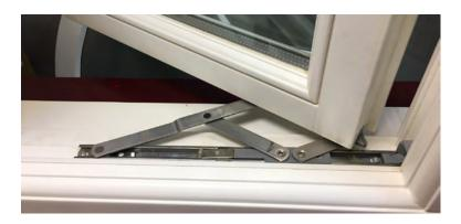
Restricted friction hinges - with child resistant button release to restrict window opening to maximum of 100mm.
