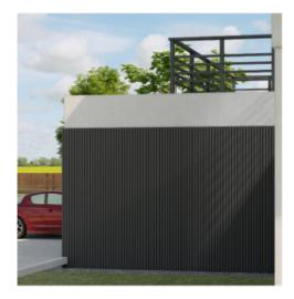
Castellated cladding panels are added to your structure either vertically or horizontally, depending on your required design.
