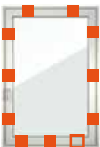
Multiple additional safeguards around perimeter
