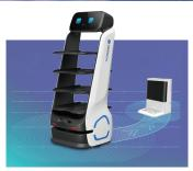
**Self charging** Configure the robot's operating hours so it autonomously returns to recharge after shifts, for reliable operation.
