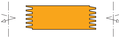
Profile 1 with continuous finger jointing
