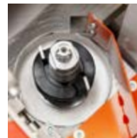
Side cutterhead For moulding and profiling
