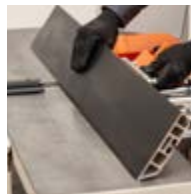
Material Guide Bar With the angle adjustment
