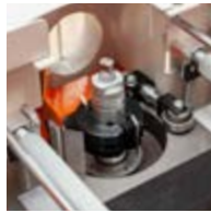
Side cutterhead For moulding and planing up to 100 mm.
