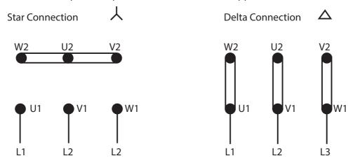
**Fig. 1** above shows a typical motor terminal arrangement for the star configuration. Three terminals are linked together with a set of three brass/copper links. The other three terminals (commonly marked U1, V1 and W1) are then connected to the three phase 415v supply (L1, L2 and L3).
