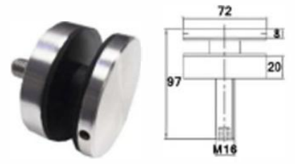
JK-1016 Solid Threaded Body - Flat Head M16 Removable Thread 304/316
