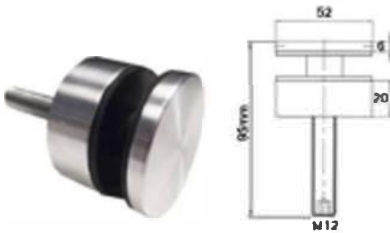
JK-1015 Solid Threaded Body - Flat Head M12 Removable Thread 304/316
