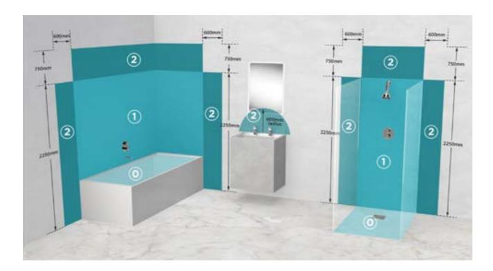
Using electrical equipment in bathrooms or wet rooms requires attention to safety. The IEE Wiring Regulations (18th Edition) have identified particular zones within the bathroom to indicate what type of electrical equipment can be installed.
