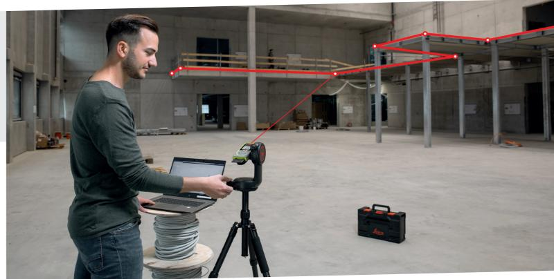
P2P Technology is a safe, accurate and efficient measurement method when it comes to distance measurements in inaccessible areas or complex measurement situations. It also enables a completely digital workflow, as the captured measurement results can be further processed in any CAD software.
