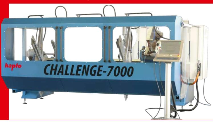
For industrial scale manufacture and to satisfy highest demands on presision and in case of extremely complexe parts, the CHALLENGE-7000 presents all technical advantages, which are characteristic for an efficient all-automatic CNC wood turning lathe. The CHALLENGE-7000 is capable of turning, milling, grooving, graving, drilling and grinding.
