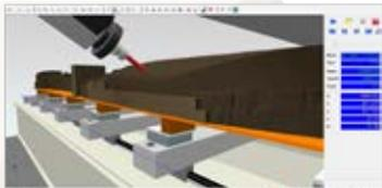
Graphic 3D simulation of the machining process and machining centre 3D collision detection                                                                |      | ○        | ○        | ○       |
