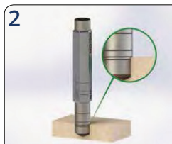
2 Verify hole diameter using Go/No-Go gauge. Check hole depth against reference line on Go side of gauge.
