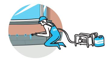
E.g.: the consumption for a wall of 5 m long and 20 cm thick will range from 15 to 20 L.
