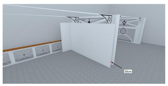
This is a diagram showing the dimensions of a 1m wide x 2.74m high wall panel including the location of the wooden batten frame which is where you can put pins, nails etc.
