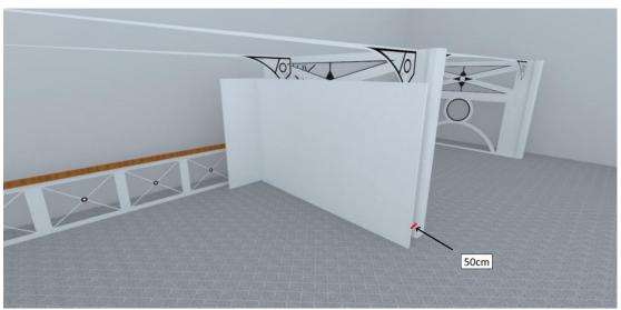
This is a diagram showing the dimensions of a 1m wide  $\times$  2.74m high wall panel including the location of the wooden batten frame which is where you can put pins, nails etc.
