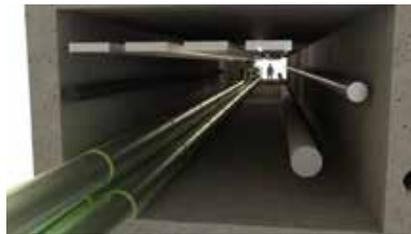
Hivoduct uses highly conductive aluminium pipes with large conductor cross-sections of up to 5,000mm<sup>2</sup>. At a nominal voltage of 245kV, a single system already allows a power transmission up to 1,600MW and, compared with conventional overhead lines, losses per kilometre are up to five times lower. The product portfolio covers the complete range from medium- to high-voltage (12kV to 420kV) and all current ratings up to 5000A.
