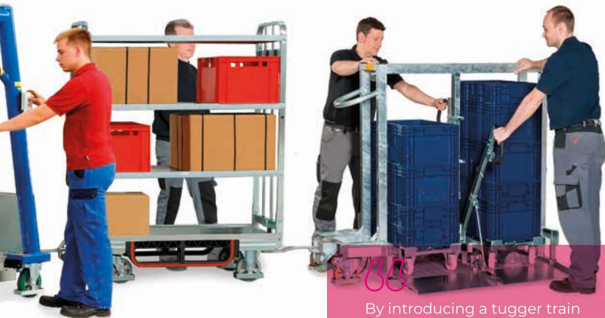
By introducing a tugger train system into an operation, companies are now able to transport a greater volume of material and they can therefore decrease the frequency of deliveries. For example, five pallets towed using specialist trolleys versus one pallet moved with a forklift or powered pallet truck. The obvious advantages being time and cost savings, and by reducing the volume of material handling equipment on site, employee safety is thereby greatly improved.
