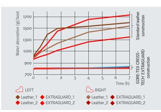
Compared with conventional fire boots, GORE-TEX CROSSTECH® EXTRAGUARD boots have very low water absorption, confirmed by the water bucket test.
