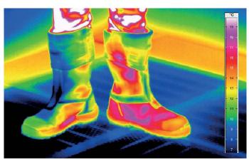
Conductive heat loss of a GORE-TEX CROSSTECH® EXTRAGUARD boot is considerably less than that of an identical leather version.
