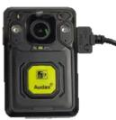
At just 38 grams, the Audax® Mini Cam is capable of capturing 1080p HD video and, unlike other cameras, also has both manually selectable and auto Infrared lights for night vision.
