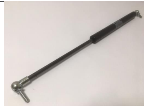
AP part no: DUC-0080-ST Rear Door Closure Kit Gas Strut (fits 270 degree hinge vehicles)
