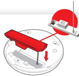
Simply plug in Ei3000MRF SmartLINK module for wireless interconnection between alarms and to communicate with the Ei1000G SmartLINK Gateway
