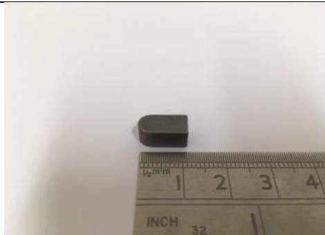
AP part no: RMP-0170-BO 12mm Key (Passive axle) Bin No. 9172a
