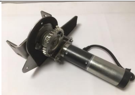
AP part no: RMP-0141E-VA** Fiat Complete Active Side Drive-gear Unit (gear drive – October 2020 onwards)
