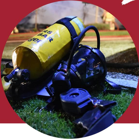
It is crucial for tackling fires safely in buildings, providing firefighters with protection from death, injury and disease when working in oxygen-deficient, toxic and hazardous atmospheres.
