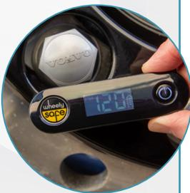
These handy tools are the perfect way to speed up fleet inspections for workshop staff, providing access to instant tyre pressure readings in either Bar or PSI when held next to any Wheely-Safe TPMS sensor.
