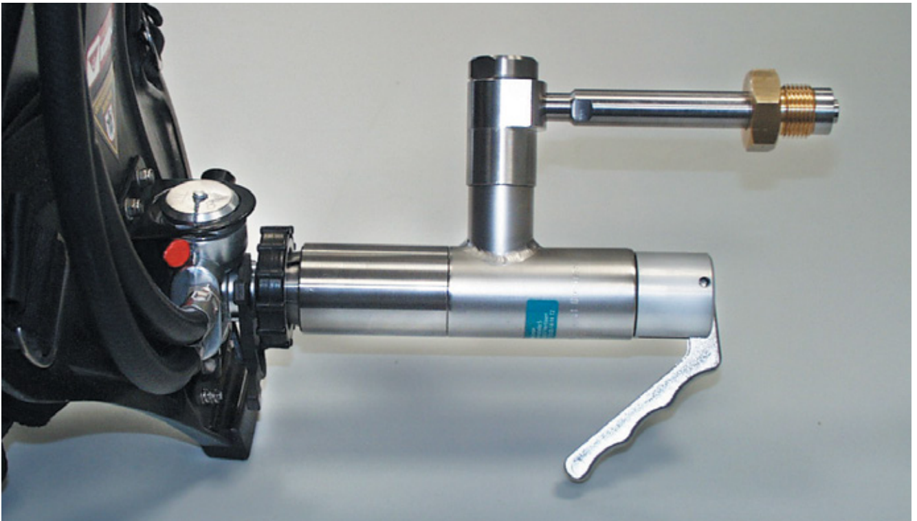
Testing of respiratory equipment with TW156 quick connector
