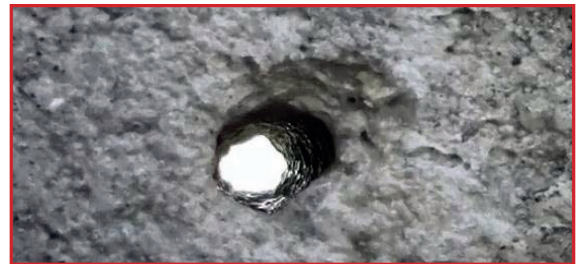
Concrete thickness: 130 mm. Drilling time: 31 sec. Cement thickness: 210 mm. Drilling time: 1 min. e 10/20 sec.
