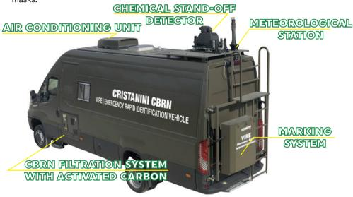
Though not primarily designed to operate within the contaminated area, this is possible due to the COLPRO system integrated to protect the operators without the need for overpressure.
