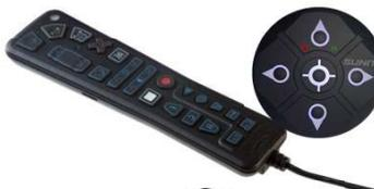
**SUNIT Hand-held Keypad.** 24 or 5-button pad for registry of Events, Average Speed-measuring's, Camera-settings, etc.
