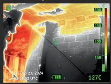
It's intuitive colorization. Kicking in at 260° C (500° F), this color threshold visually alerts fire-fighters when temperatures approach a range that may begin to damage personal protective equipment. Consistent and transparent color scheme for quick scene assessment.
