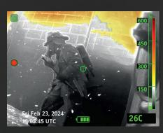
**Seamless operation.** No forced shuttering when transitioning between hotter and cooler areas of a scene.
