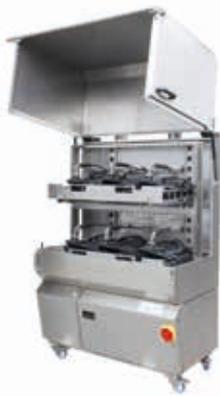
The professional washing machine Harstra Wash6DR is an allrounder for the cleaning of PPE such as SCBAs, face masks, lung demand valves, and helmets. The machine has been a joined development between Dräger and the Dutch cleaning equipment manufacturer Harstra.
