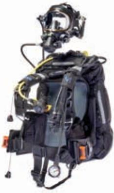
The PSS® Dive is a combination of a carrying and buoyancy system, approved according to EN 1809, for professional diving use. It can be individually configured with various components, such as the Panorama Nova Dive full-face mask and the Secor 7000 pneumatic system. The PSS Dive is approved for diving with single or double cylinders.
