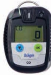
The robust Dräger PAC® 6500 is your reliable companion under tough conditions. The personal single-gas detection device warns against hazardous concentrations such as carbon monoxide with precision and reliability.
