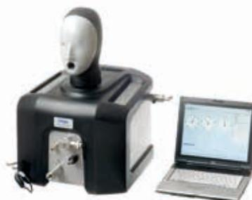
All static and dynamic tests of the Dräger Quaestor 7000 are carried out fully automatically. For the user this guarantees high efficiency through comfort and speed.
