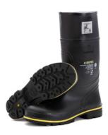
A heat-resistant safety boot conforming to the EN 15090  $\rm HI_3$  F3A fire boot standard for flame resistance, radiant heat (20kW/m²) and heat insulation of the sole (250°C for 40 minutes). These boots are designed for use in areas where there is a risk of sparks from welding or grinding or for close proximity fire fighting.
