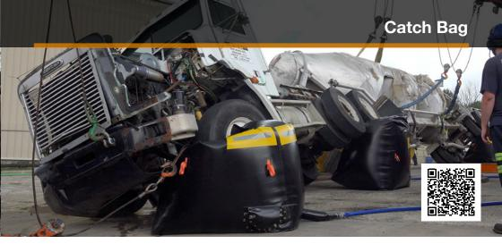
Catch Bags are designed to be used in conjunction with our High Lifting Bags during the uprighting of vehicles or objects. The Catch Bags prevent a rapid and dangerous decent which prevents further damage to the vehicle or object being lifted and allows for a safer environment for the recovery team.
