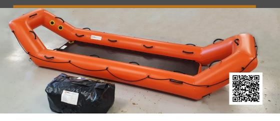
The RSW Rescue Sled is fitted with extended tubes which provide its unique design. Based on the design of the standard Rescue Sled, it provides options for rescuing casualties from difficult situations such as weirs. Its design allows casualties to be pulled aboard through the wrap round tubes, which provide protection and also stability when in the water.
