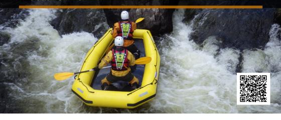
Fully inflatable, the Evacuation Raft is lightweight and portable. It is easy to manoeuvre, and can be paddled or pulled by hand. The Evacuation Raft has a flat bottom, making it exceptionally stable and suitable for use in very shallow water from 50mm in depth. The Evacuation Raft is ideal in flood rescue situations.
