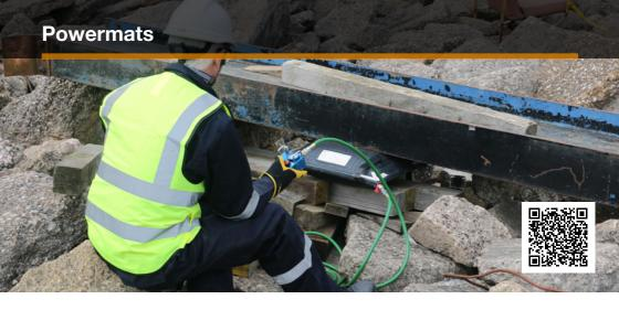
The Powermat is a heavy duty, high pressure lifting bag designed primarily for lifting vehicles and objects in emergency situations. Deflated, the Powermat has a very slim profile making it suitable for use in restricted or awkward spaces and compact to store. Available in 12 standard sizes with maximum lifting capacities from 1 tonne right up to 68 tonne.
